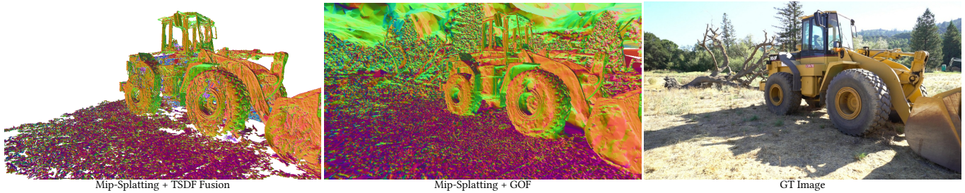
Fig. 8. Comparison of mesh extraction methods. Applying GOF to SOTA Mip-Splatting [Yu et al. 2024a] yields significant improvements over TSDF, enabling complete mesh extraction for background regions.
