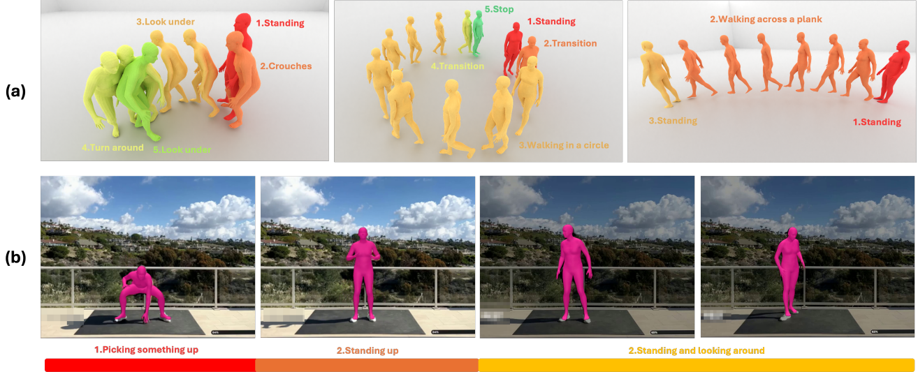
Figure 4. Motion-to-Text understanding of MoCap and YouTube data. (a) Given an input MoCap sequence, we use UniMotion to predict frame-level local text. (b) We annotate human motion from YouTube videos with frame-level text. We lift 2D videos to 3D human motion via frame-by-frame pose estimators [10]. We visualize the SMPL human pose (Pink) overlaid on the YouTube videos frames. Then we run UniMotion to predict frame-level annotations (colored text descriptions below the frames). Annotations could serve as valuable audio close captions for the visually impaired.
