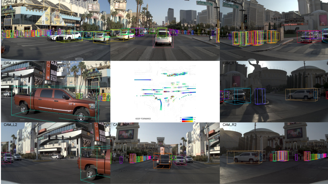
Figure 2: Visualization of the PARA-Drive Model’s output. Eight surrounding cameras are displayed with detected object bounding boxes. In the center, the predicted BEV information is shown, including object bounding boxes, their predicted multi-modal future trajectories, as well as the planned trajectory for the ego vehicle.
