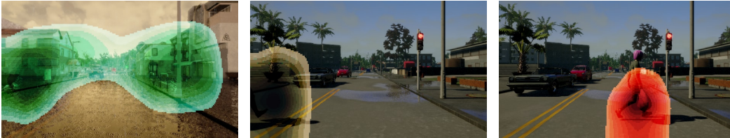
Figure 4: Attention Analysis. Left: The network focuses at the periphery for recognizing traffic lights. Middle: The network is anticipating a hazard stop by observing the shadow of a pedestrian. Right: The network focuses its attention on the pedestrian to correctly predict a hazard stop.
