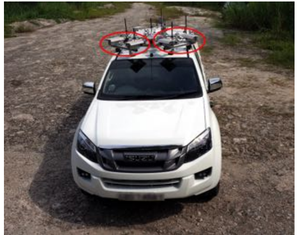
Fig. 4: DSO’s Isuzu D-Max platform equipped with two fisheye-stereo cameras which are shown enclosed in red ellipses.
