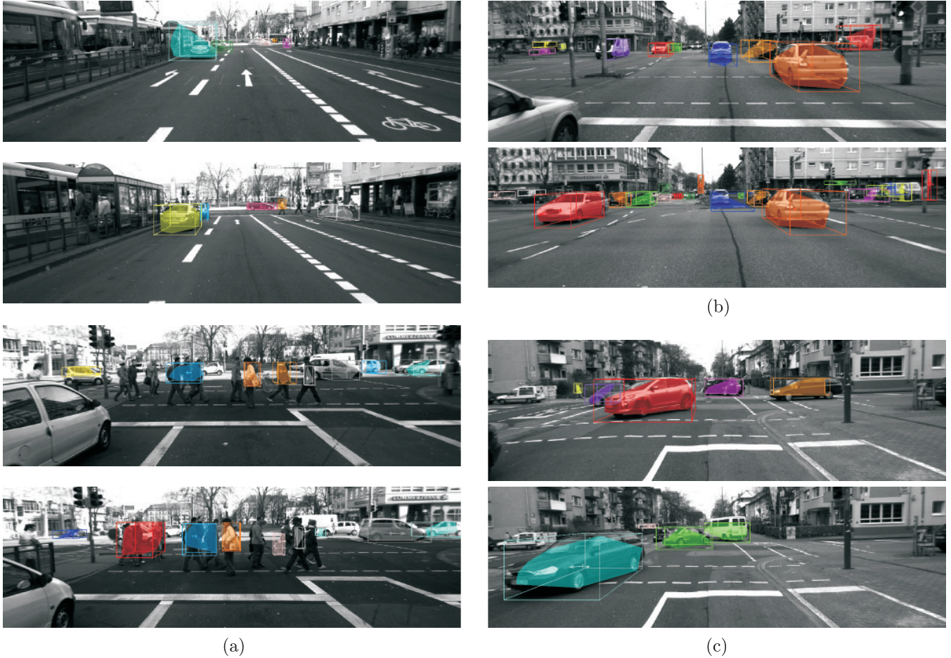
Fig. 9. Results on inner city intersections. (a) Slowly moving and small objects such as the pedestrian in the first two frames are detected in a range up to 30 m. However, the track of such a small object is interrupted and it is not continuously tracked. Similarly moving groups of pedestrians are detected as one object since the scene flow difference is not unique and the number of detected interest points is too low. (b) Moving objects in this sequence are detected, but especially for the far range static objects are detected as well. (c) Turning cars and partly occluded objects, which were fully visible and observed in a previous frame, are detected. Since continuous velocity is assumed, the Observation-to-Track association fails for sharply turning objects.
