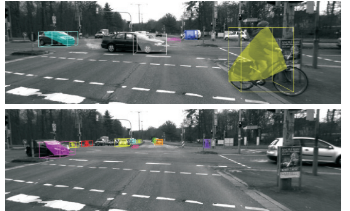
Fig. 8. Results on a rural intersection. Close range objects as the cyclist or the crossing traffic in the first frame are detected as well as objects in the far range in the second frame.
